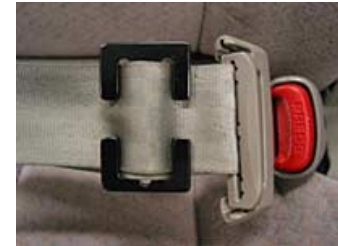
Figure 3: Combination Lap/Shoulder Belt with Locking Clip
